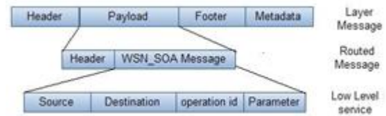
Fig 3: Message structure in the low level SOA in WSN
