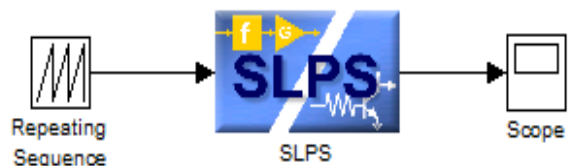
Fig 2: Co-Simulation Model in Simulink using SLPS Block
