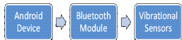
Fig 2. Interfacing of Android device to vibrators via Bluetooth
