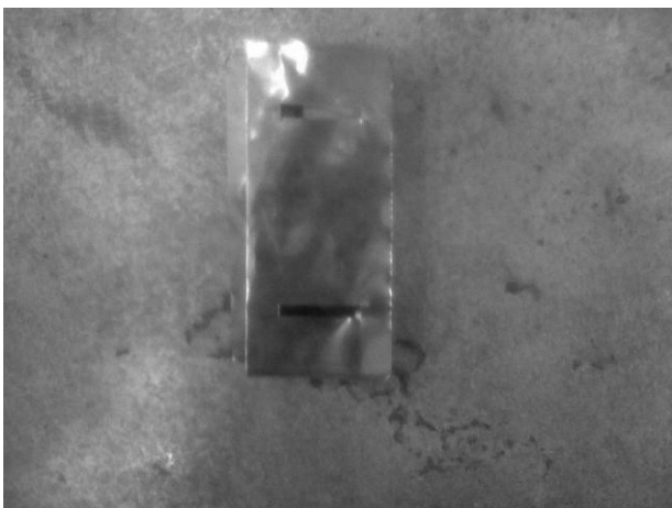
Fig 9: Fabricated prototype of shorted plate pair of rectangular slots cut proximity fed MSA
