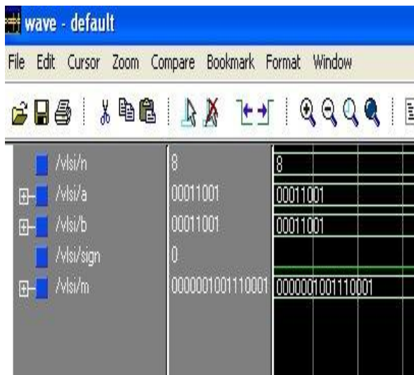
Figure 5. Simulation result for 8 bit unsigned multiplication
