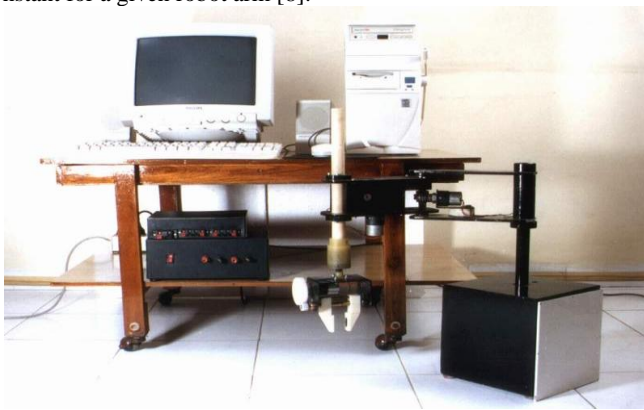
Fig. 4. The computer controlled SCARA robot
