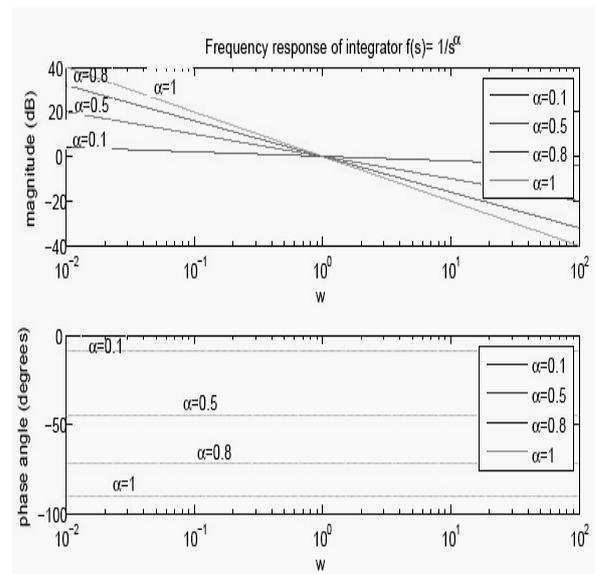
Fig. 2. Frequency response of Example (1) for different values of  $\alpha$
