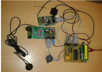
Fig 2 The Hardware Setup for VTS
