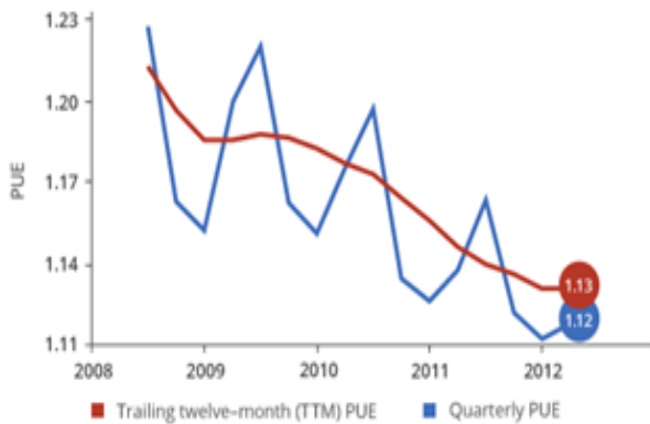
Figure 5: Graph shows continuous improvement of Energy efficiency in large Google datacenters (Source: Google.com)
