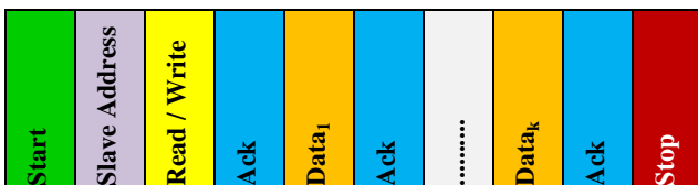
Figure 2: Frame format of I 2 C Protocol
