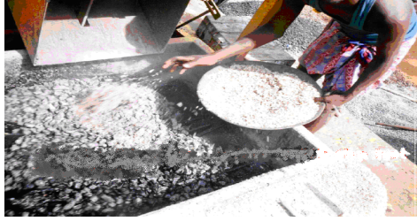
Fig 7: Shredded plastic waste is added
