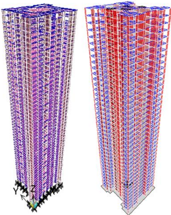
Fig 2: Etabs 3D view of model with (i) Fixed support (ii) Support on raft
