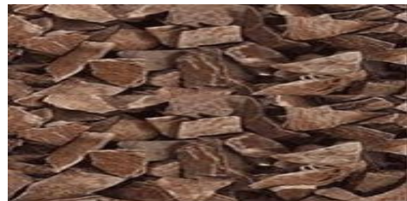
Fig 2: Coconut Shell as aggregates
