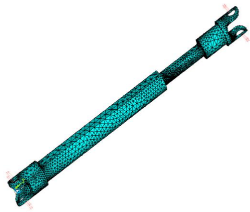
Fig.3. Meshed view with loads applied
