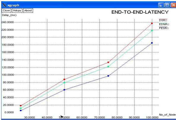
Figure 4. This result shows us that PESR has a low Delay than the DSR & EDNR protocols.
