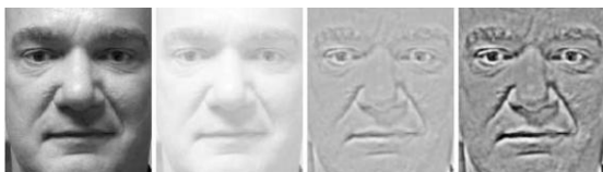
Fig. 2. (Top) the stages of our image preprocessing pipeline, and (bottom) an example of the effect of the three stages—from left to right: input image; image after Gamma correction; image after DoG filtering; image after robust contrast normalization.
