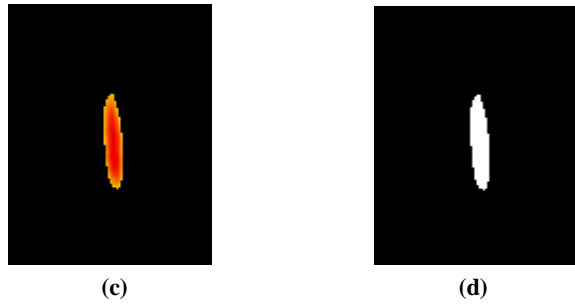
Figure 11: (a) Original Rectangular Notch Image. (b) filtered image. (c) K-means Segmented defect region. (d) threshold image.
