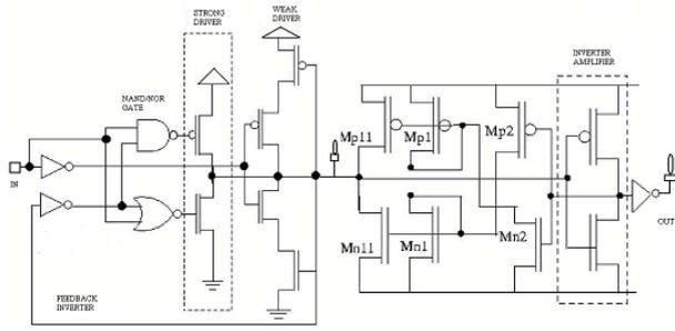
**Fig 1: CMS scheme with driver pre-emphasis- CMS-Fb circuit**
