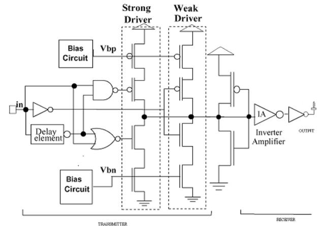
**Fig.3: Proposed current-mode signaling scheme (CMS-Bias)**
