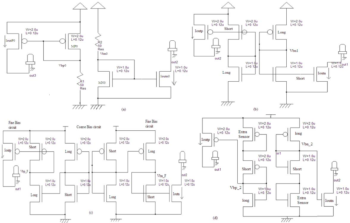
**Fig. 4: Derivation of the proposed corner-aware bias circuit. a) Resistance based; b) diode-connected transistor based; c) two step (fine-coarse) compensation; d) diode-connected devices with extra sensor.**
