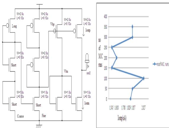
**Fig 5(a) Proposed corner-aware bias circuit (b) probability density function of output curve**
