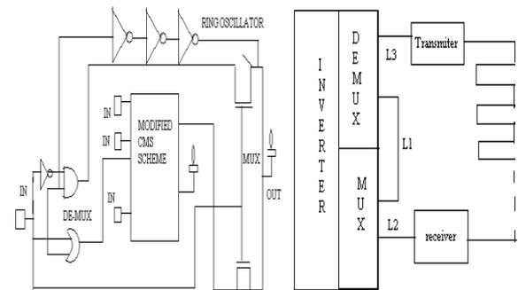
**Fig 7(a): Delay Measurement Scheme Using Modified Smart Bias CMS Scheme (b) Block Diagram Of Delay Measurement Scheme**
