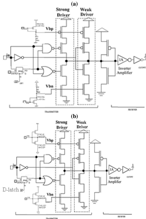
**Fig 6 (a): Modified Smart Bias CMS Scheme D-latch with resistance circuit (b) Modified Smart Bias CMS Scheme with terminating inverter**
