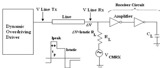
**Fig 2: Macro model of dynamic overdriving CMS scheme**
