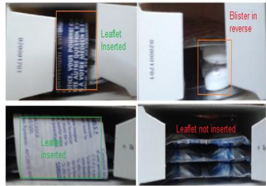
Fig 7: Leaflet inserted correctly (Top left); Blister missing and one Blister turnout side down (Top right) Leaflet inserted (Bottom left); Blisters correctly inserted, but leaflet missing (Bottom right)
