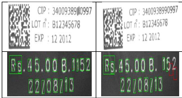
Fig. 9: Data Matrix decoder and OCR usage to test readability of label on carton
