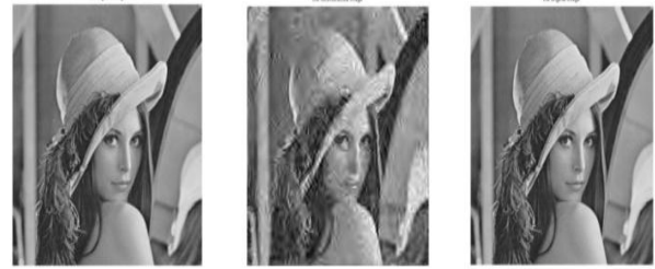
Fig 5: The decoded “LENA” from left to right, (a) original, (b) Original OFDM [PSNR= 24.5140 dB], (c) Modified OFDM (UEP) [PSNR=30.4160 dB]
