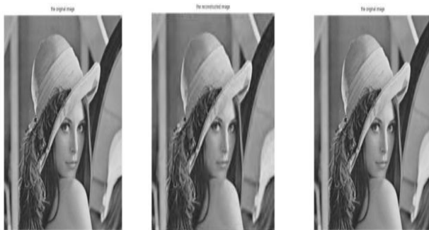
Fig7:The decoded “LENA” from left to right, (a) original, (b) modifiedOFDM [PSNR= 30.4160 dB], (c) Modified OFDM with adaptive clipping[PSNR= 29.5970 dB] over AWGN
