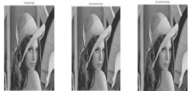
Fig9: The decoded “LENA” from left to right (a) original (b) modifiedOFDM [PSNR= 30.4160 dB] (c) Modified OFDM with adaptive clipping [PSNR= 29.9306 dB] over AWGN channel at SNR=15 dB with QAM16
