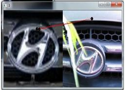
Fig 3:Matching points found for a given template image and the input frame
