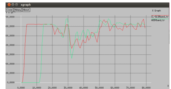
Figure 7: Bandwidth analysis of CL-OLSR and AODV protocols
