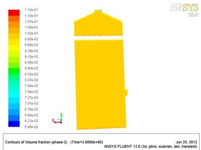
Fig. 5. Volume Fraction of dust concentration of Wet scrubber.
