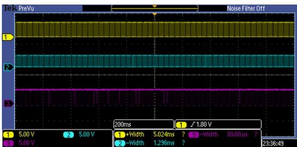
Fig. 9 Output of ZCD (Ch#1), output of OS (Ch#2) and output of gate G-1 (Ch#3) in Roll Mode at 200 ms.
