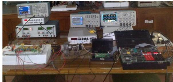
Fig. 11. Experimental setup for the measurement of velocity of vibrations.
