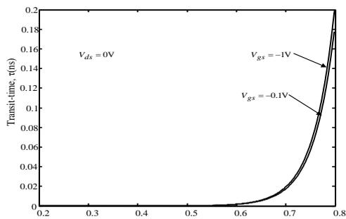
**Fig. 3. Variation of transit-time with gate-length for different gate-source voltages**
