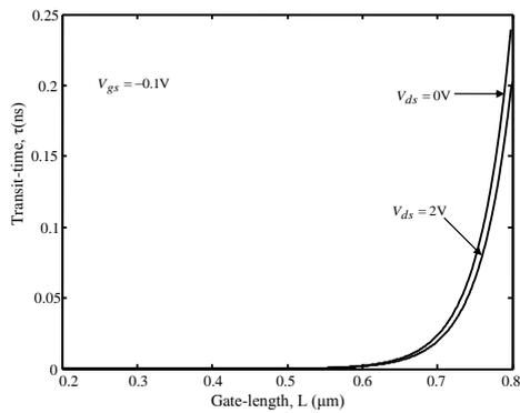
**Fig. 2. Variation of transit-time with gate-length for different drain-source voltages**
