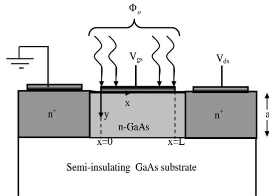
**Fig. 1. Schematic of GaAs OPFET used for the modeling.  $a$  is the thickness of active channel region,  $L$  is the length of the Schottky metal gate and  $\Phi_o$  is the incident flux density**
