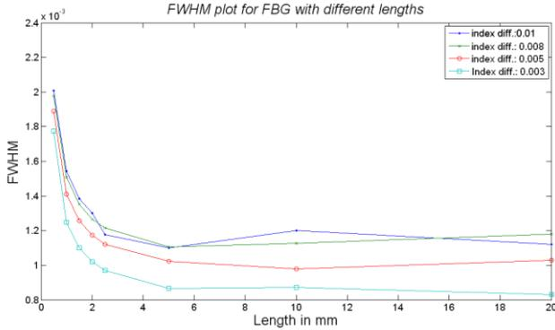
Fig. 5. Relationship between FBG bandwidth and grating length
