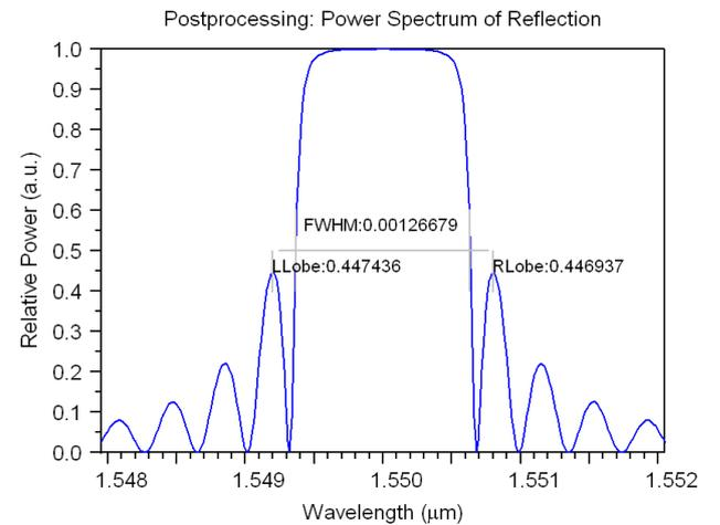
Fig 4. Grating Spectral Response for  $L=2mm$ , Index diff.: 0.008
