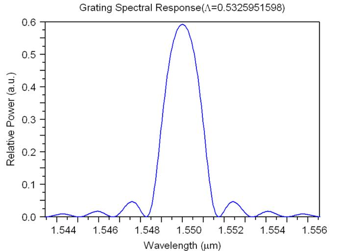
Fig 3. Grating Spectral Response for  $L=0.5mm$ ,  $\Delta n_0:0.008$
