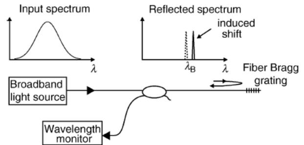
Fig 1. Basic reflective FBG sensor system
