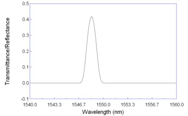
Fig. 6. No chirp, Length: 1.0 mm, Apodization Raised Cosine
