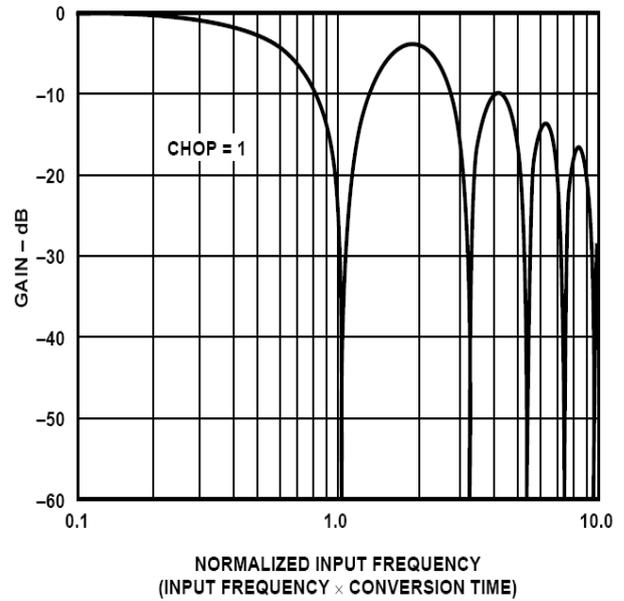
Fig 4: ADC Frequency Response, Chopping Enabled
