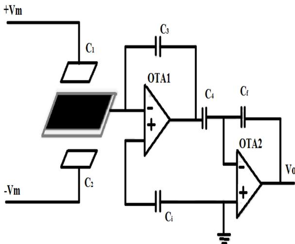
Fig 1: schematic of the self balancing capacitor bridge
