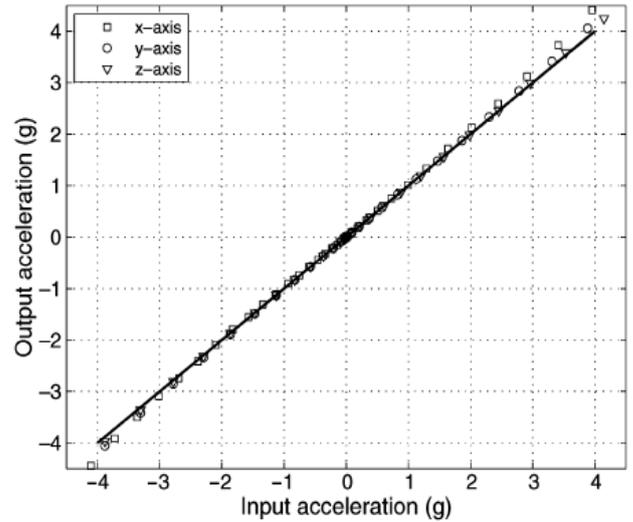
Fig 6: Measured dc acceleration in x-, y-, and z-directions.
