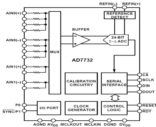
Fig 3: Block diagram of AD7732 sigma-delta chip
