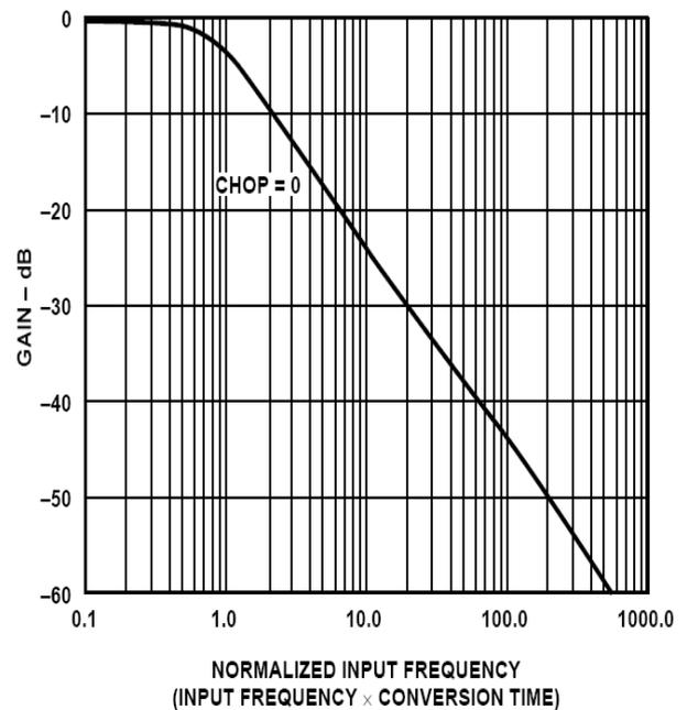
Fig 5: ADC Frequency Response, Chopping Disabled
