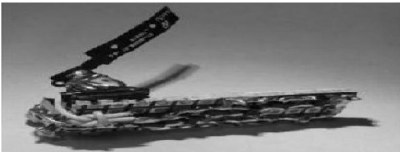
Fig: 8 Based on case 4, the proposed three-stage Villard voltage multiplier with film-typed antenna
