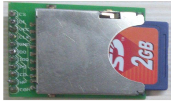
Fig 3: Pins of the SD Card Breakout
