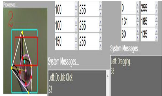
Fig 6(a): Left Double click and Drag Operation Detection
