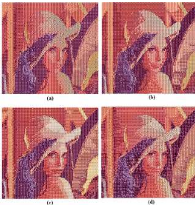
Figure 1 Reconstructed Images using LBG algorithm for lena Image with different codebook size (a) Codebook size=128,(b) Codebook size =256, (c) Codebook size =512, (d) Codebook size =1024
