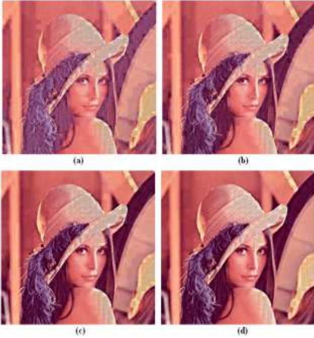
Figure 3 Reconstructed Images using An Improved LBG algorithm with DCT for lena Image with different codebook size (a) Codebook size=128,(b) Codebook size =256, (c) Codebook size =512, (d) Codebook size =1024
