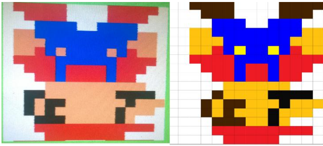
Figure 9: 180° Rotation On FPGA (left) and MATLAB(right)
