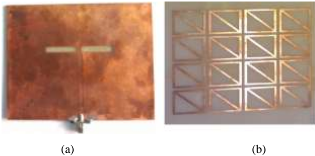
Fig 3: Photograph of CPW-fed slot antenna with metasurface (a) Top View and (b) Bottom view
