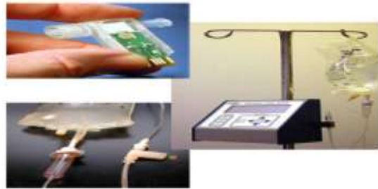
Fig 6: Drug infusion monitoring using micro coriolis flow sensor.
