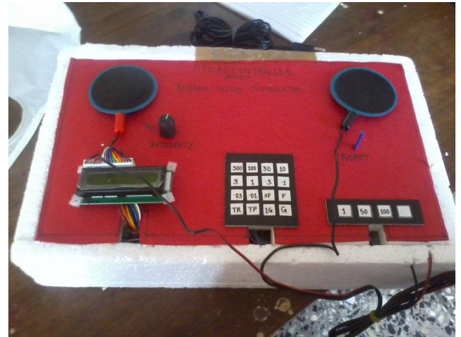
Fig.8 Microcontroller based Rehabilitation Stimulator
