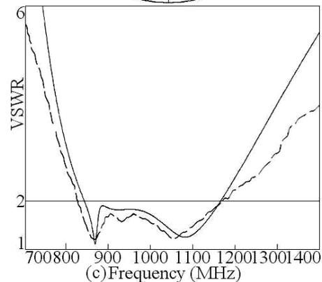
**Fig. 4 (a, b) Surface current distribution at dual peaks and (c) input impedance and VSWR plots, (—) simulated, (— —) measured, for optimized proximity fed gap-coupled C-shaped MSAs**
