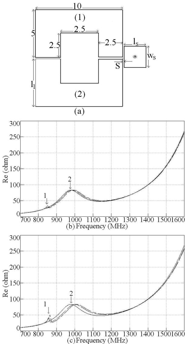
**Fig. 3 (a) Proximity fed gap-coupled C-shaped MSAs and its resonance curve plot for ' $l_1$ ' = (b) (—) 5.0, (— —) 4.8, (— — —) 4.6, (c) (—) 5.0, (— —) 4.8, (— — —) 4.6**
