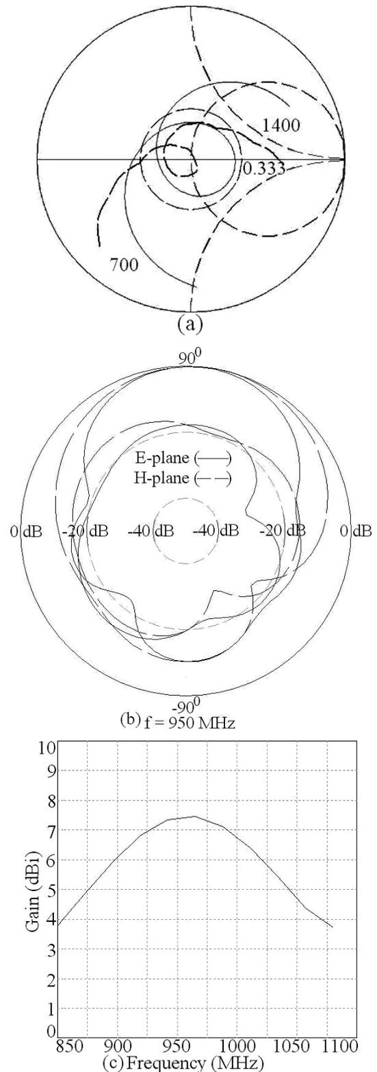
**Fig. 2 (a) Input impedance plots, (—) simulated, (---) measured, (b) radiation pattern at center frequency and (c) gain variation over BW for proximity fed C-shaped MSA**
