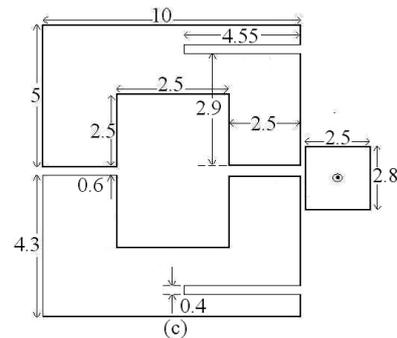
**Fig. 6 (a) Gain variation over BW and (b) fabricated prototype of proximity fed gap-coupled C-shaped MSAs and (c) proximity fed gap-coupled rectangular slot cut C-shaped MSAs**
