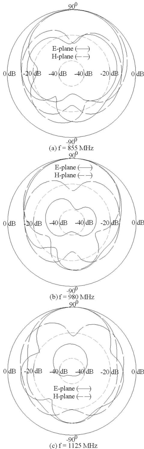
**Fig. 5 (a – c) Radiation pattern over the BW for proximity fed gap-coupled C-shaped MSAs**
