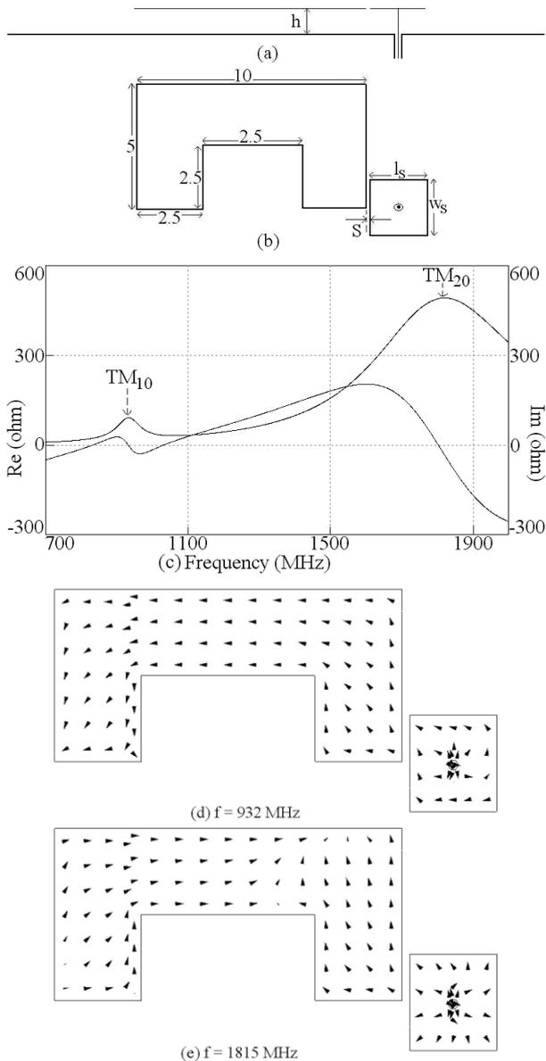
**Fig. 1 (a) Top and (b) side views of proximity fed C-shaped MSA, its (c) resonance curve plot and its (d, e) surface current distribution at dual peaks**
