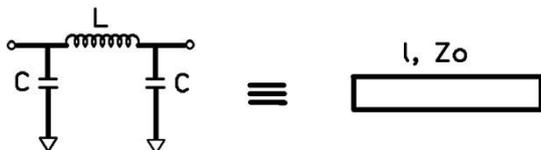
Fig.2.  $\Pi$  network equivalent for a transmission line
