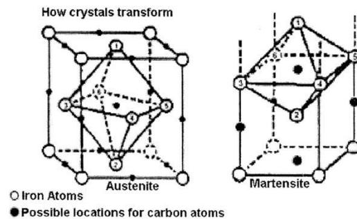
Fig.-12 Transformation of retained austenite to martensite
