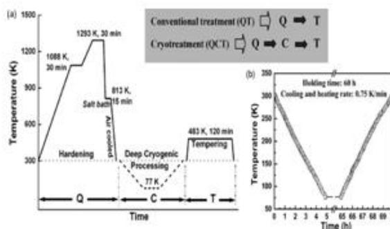
**Fig.2. (a) Schematic representation of the heat treatment schedule consisting of hardening (Q), deep cryogenic processing (C) and tempering (T) cycles, and (b) typical time-temperature profile of a deep cryogenic processing cycle**
