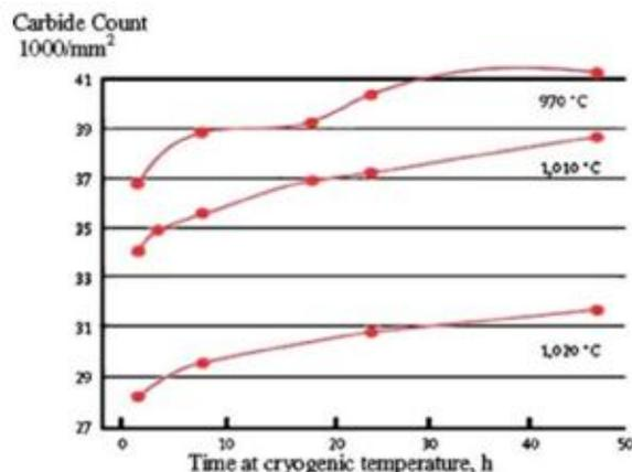
Fig.-5 Effect of soaking period at  $-196^{\circ}\text{C}$  ( $-320^{\circ}\text{F}$ ) on carbide number for D2 steel. Carbides were measured using optical techniques. Austenitizing temperatures of  $970^{\circ}\text{C}$ ,  $1,010^{\circ}\text{C}$ ,  $1,040^{\circ}\text{C}$ , and  $1,070^{\circ}\text{C}$  were used before hardening [
