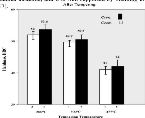
**Fig. 9- Hardness for different tempering temperatures after cryogenic and conventional treatments**
