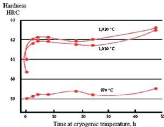
Fig.-6 Effect of austenitizing temperature and holding time at cryogenic temperature on hardness of D2 cold-work tool steel
