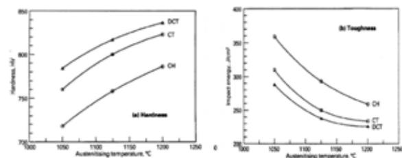
Fig.-13 Effect of austenitizing Temperature and Cold Treatment on a) Hardness and b) Toughness Where, CH–conventional heat treatment CT–Cold treatment DCT-Deep cryogenic treatment
