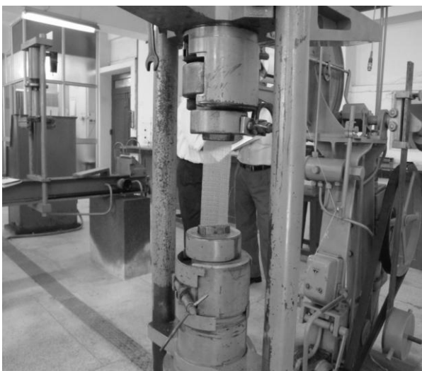
Fig. 3 Strip tensile test of geotextile
