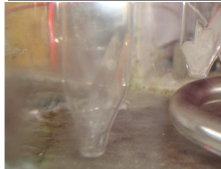
Photograph showing grown crystal KDP
