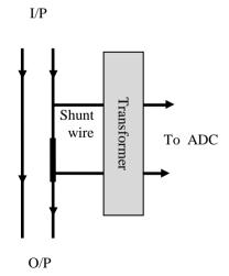
Experimental Arrangement of current sensing
