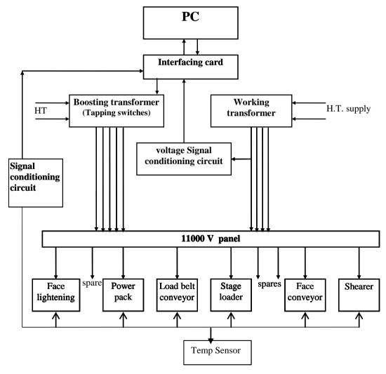
Fig.1 block diagram of the power management system of long tunnel face
