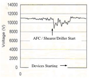
Fig. 7 Graph of Voltage drop with device starting
