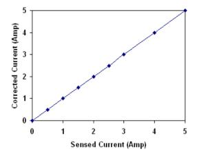
Fig. 5b: Measured Current Versus Sensed Current
