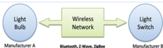
Fig 1: Device to device communication model
