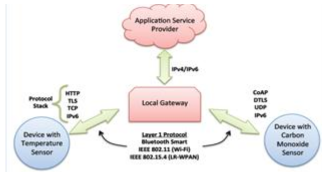
Fig 2: Device to gateway communication model
