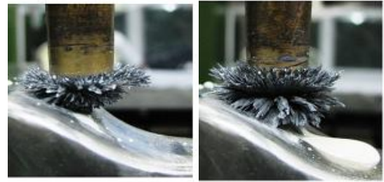
Fig.7. Condition of MR fluid brush at different rotational speed of tool 900 RPM and 1100 RPM respectively [11]
