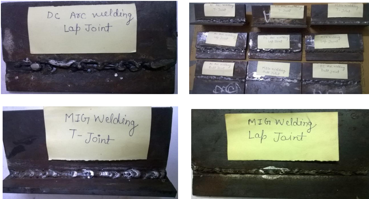
Fig 3: Welded joints considered for experiment
