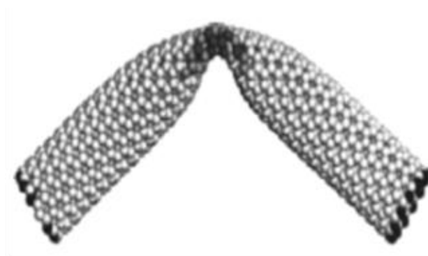
Fig 2: Transverse deformation of a carbon nanotube (Computer simulation), as adapted from [11].
