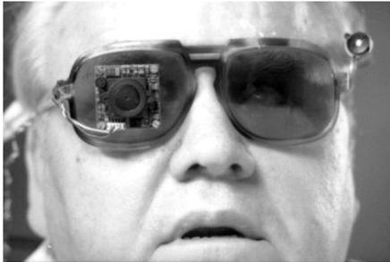
**Figure2.** Blind volunteer with sub-miniature TV camera mounted on the right lens of his sunglasses, and the laser-pointer (position monitor) on the left temple piece.
