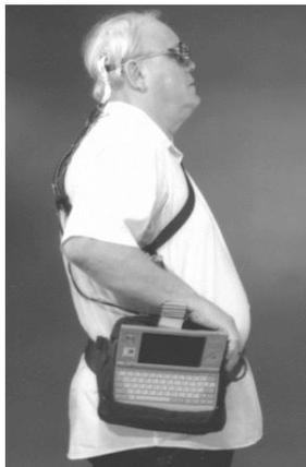
**Figure3.** Complete artificial vision system that contains a computer and other electronic packages connected with the electrodes to eye.
