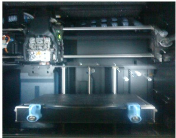
Figure 4 : Fused Deposition Modelling Machine
