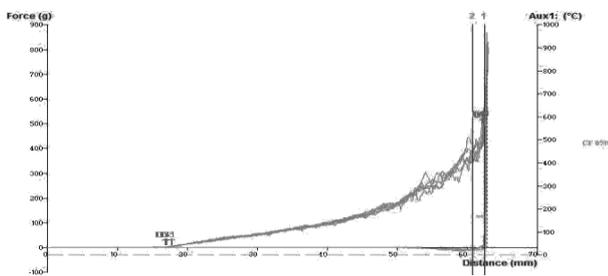
**Fig. 3: Caking Strength of the commercial rice flour**
