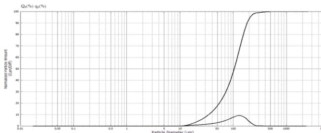
Fig. 1: Particle size analysis of commercial rice flour
