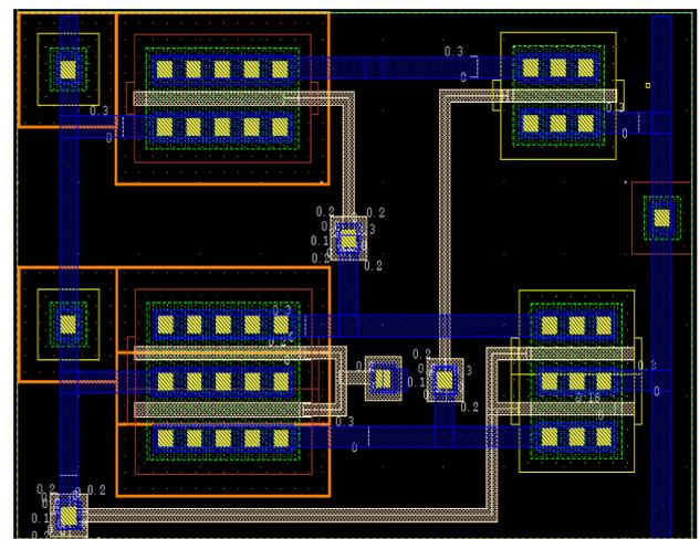
**Fig. 10 Layout of current sink logic structures based Schmitt trigger**
