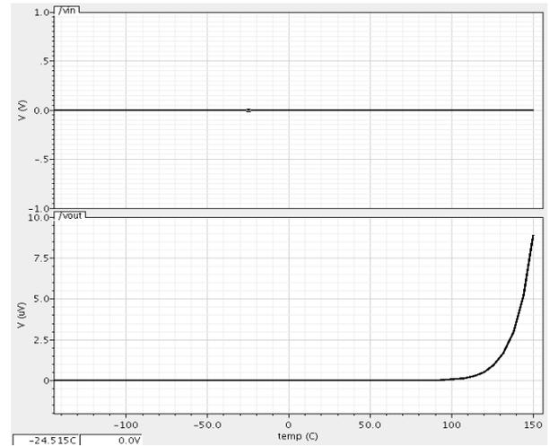
**Fig. 8 Temperature sensitivity characteristics of the proposed circuit of Fig.3 (above: input sine wave and below: output square wave)**
