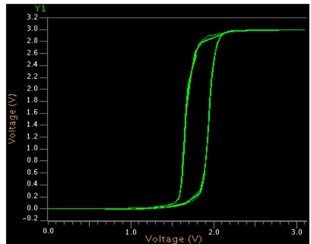
**Fig. 9 Hysteresis curve of pseudo logic structures based Schmitt trigger**
