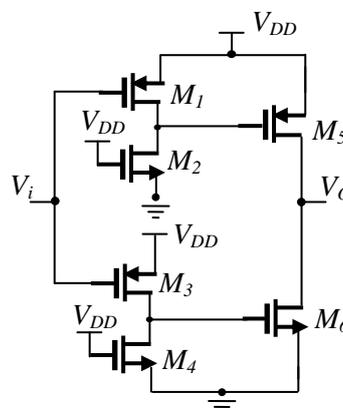
Fig. 1 Current Sink logic structures based Schmitt trigger
