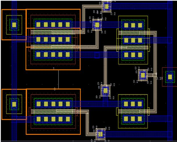
**Fig. 11 Layout of pseudo logic structures based Schmitt trigger**
