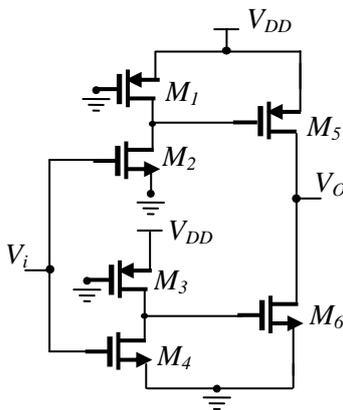
Fig. 3 Pseudo logic structures based Schmitt trigger
