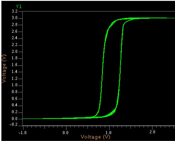
**Fig. 6 Hysteresis curve of current sink logic structures based Schmitt trigger**
