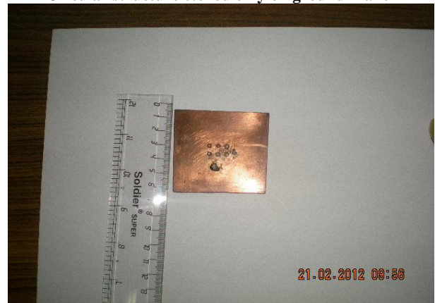
Fig X. Annular ring antenna with periodic lattice of annular structure etched only on ground Plane
