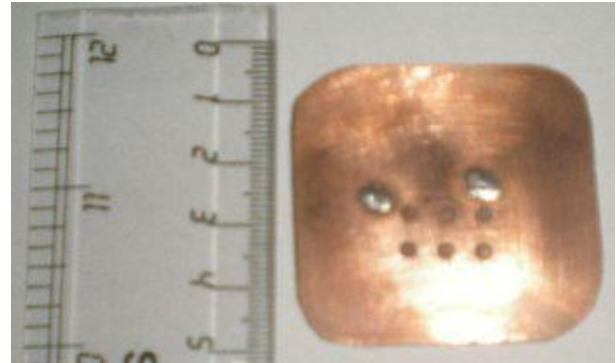
Fig IX. Annular ring antenna with periodic lattice of Circular structure etched only on ground Plane
